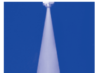
Spray pattern of the Laval nozzle
