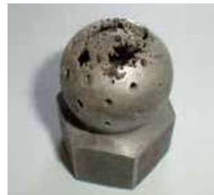
Figure 18: Chemical corrosion of a spray ball
