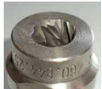
Figure 19: Wear of a full cone nozzle
