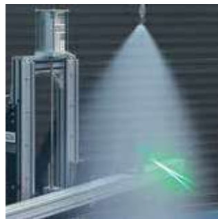
Figure 13: Droplet size measurement
