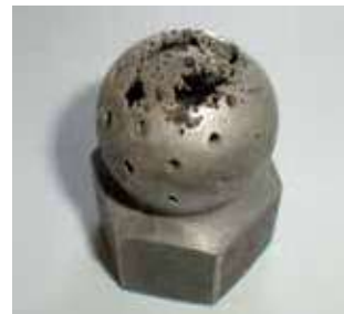
Figure 18: Chemical corrosion of a spray ball
