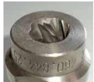
Figure 19: Wear of a full cone nozzle
