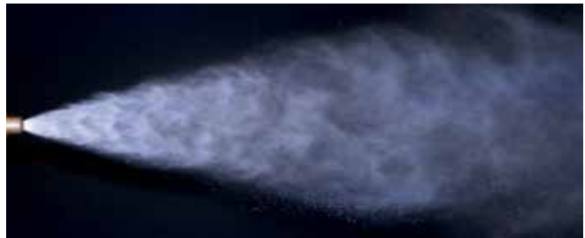
Spray pattern of the MasterNOx nozzle 30°
