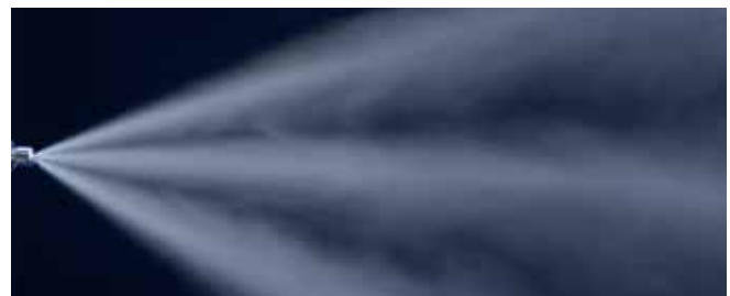
Spray pattern of the flat fan nozzle
