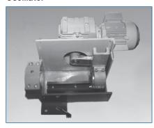
Oscillator with electromechanical crank drive for side-to-side movement by a sliding block and axial guide rail.
