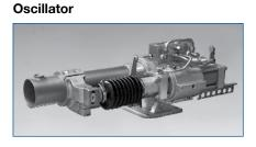
Oscillator with oil-hydraulic drive with infinitely adjustable stroke speed provided by micro-flow control valve.
