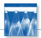
Designed specifically for STAMM® shower headers, these nozzles can serve as replacements or to change the flow rate of an existing unit. Self aligning when used with STAMM® or Lechler bases. 317 LN stainless steel construction for long service life. Available in 60°, 30°, and 15° flat fans or 0° solid stream ("needle jet") versions.
